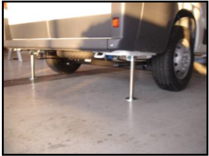
Hydraulic landing legs prevents sagging when loading and unloading cargo.
