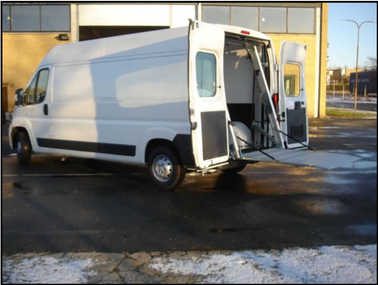
The INSIDER lift is protected against the weather as it is mounted 'indoors'.
