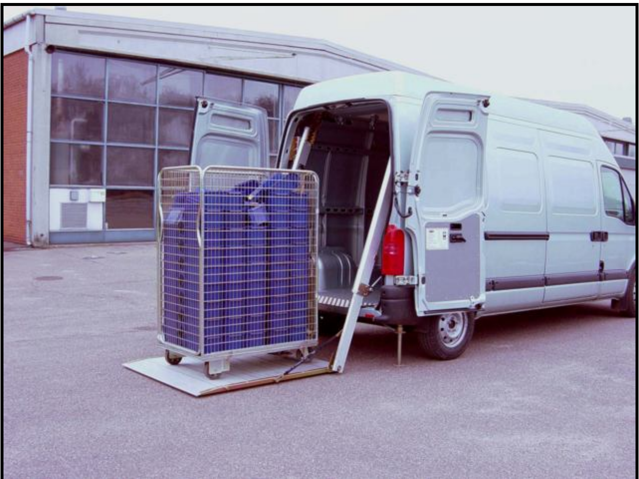
Ultra low approach angle (1.4 degrees) makes heavy loading/unloading very easy.
