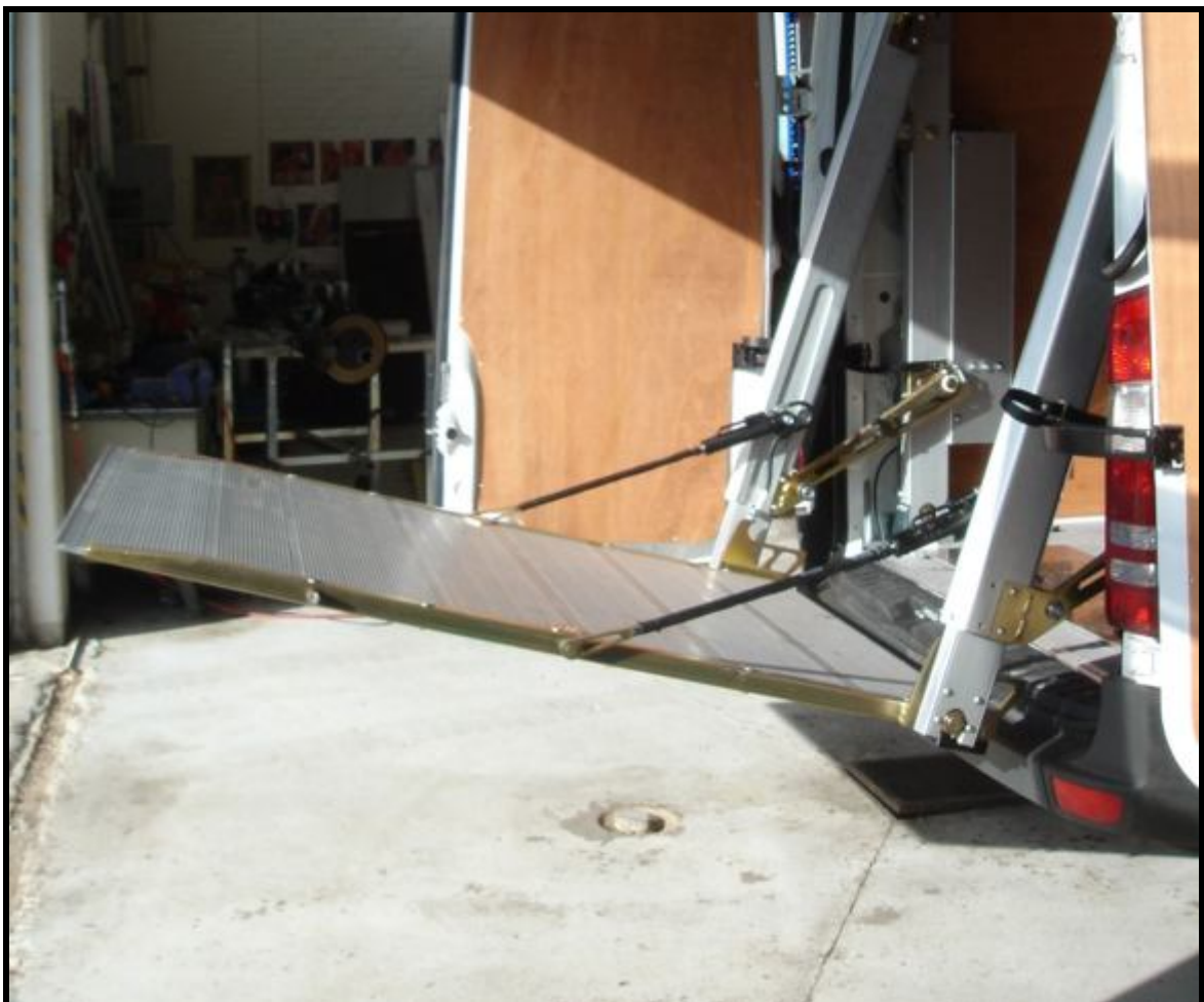
Hydraulic tilt of platform (+ 420 mm. / - 100 mm.)
